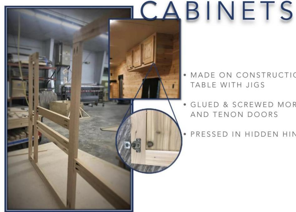
MADE ON CONSTRUCTION TABLE WITH JIGS
